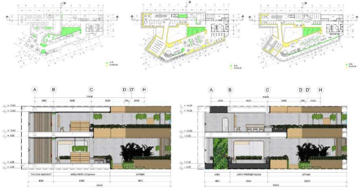
Figure 7. Distribution of Native & Artificial Plants in the Ground Plan and Elevation Drawing Source: Matthew Vincent, 2022 [8]
